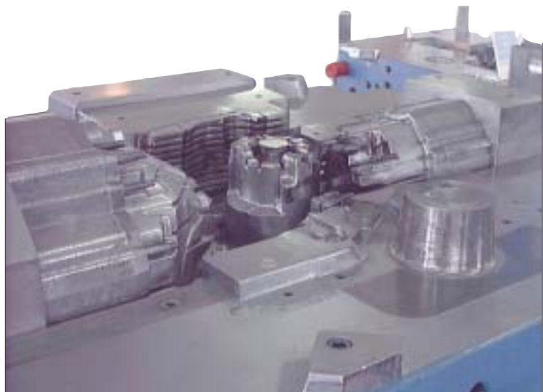
Aluminium die for the automotive industry.
