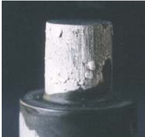
Soldering damage on a core pin.
